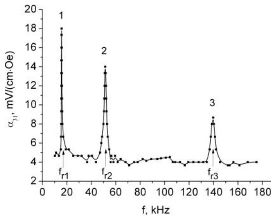
**Figure 2.** Frequency dependence of  $\alpha_{31}$  for the ME composite 0.6 TDF – 0.3 PZT at room temperature.
