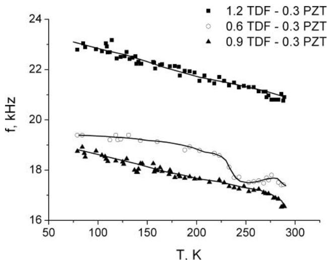
**Figure 5.** Temperature dependences of the resonant frequency  $f_{r1}$  for composites 0.6 TDF – 0.3 PZT, 0.9 TDF – 0.3 PZT, and 1.2 TDF – 0.3 PZT.
