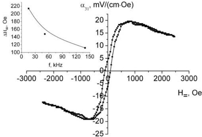
**Figure 3.** Field dependence of  $\alpha_{31}$  for the composite 0.6 TDF – 0.3 PZT at room temperature. Inset: frequency dependence of the ME hysteresis loop width  $\Delta H$  for the composite 0.6 TDF – 0.3 PZT.
