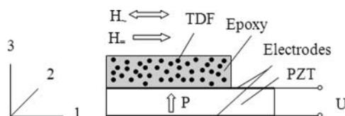
**Figure 1.** Model of composite samples of TDF – PZT and its direction in measuring  $H_{\perp}$  and bias  $H_{\parallel}$  magnetic fields.
