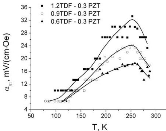
**Figure 4.** Temperature dependences of  $\alpha_{31}$  at  $f_{rl}$  for composites 0.6 TDF – 0.3 PZT, 0.9 TDF – 0.3 PZT, and 1.2 TDF – 0.3 PZT.
